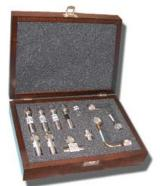
measurement accessory kit (P/N 187-4001) that is supplied as part of the system. The measurement accessory kit includes low SWR masking attenuators and a power divider to provide a measurement system as shown in Figure 1.
